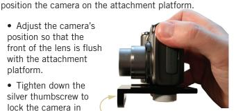
Align the camera lens with the end of attachment platform that has the three threaded holes.
