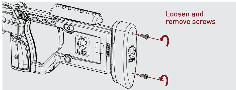
**Step 2:** Replace these screws with the longer screws, which are long enough to go through your desired amount of spacers. Insert desired quantity of spacers onto the longer screws
