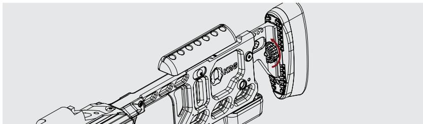
**Step 2:** Slide the buttpad up or down in 1/4" increments, or cant it 15 degrees to either side. There are protrusions on the aluminum LOP bar that fit into pockets on the polymer buttpad housing. Retighten Thumbscrew when you have it set where you want.
