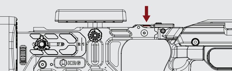
**NOTE:** The latch mechanism to hold the buttstock in the folded position is a positive lock system. You **MUST** press the unlock button pictured above to unfold the stock. It does not release just by pulling on the buttstock.
