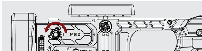
**Step 2:** Push in on the thumbscrew to disengage the LOP lock.
