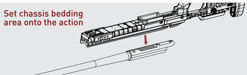
**Step 3:** Drop the middle and rear action screws into place. Turn the screws to engage the threads in the action. Again do not fully tighten. The middle action screw gets an M6 washer under the head. The rear action screw does not get a washer. For post-2013 rifles, use silver button head rear action screw. For pre-2013 rifles use black socket head rear action screw. For all rifles, insert included shim between chassis and action at middle action screw position
