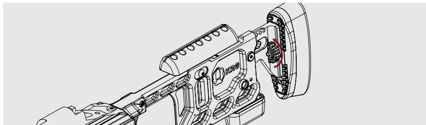
**Step 2:** Slide the buttpad up or down in 1/4" increments, or cant it 15 degrees to either side. There are protrusions on the aluminum LOP bar that fit into pockets on the polymer buttpad housing. Retighten Thumbscrew when you have it set where you want.
