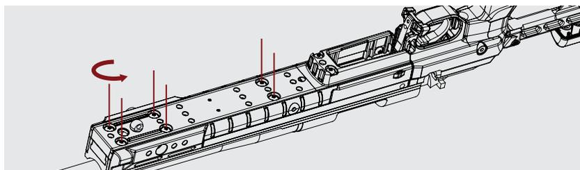
**Step 3:** If unable to achieve desired fit, trigger guard can be moved forward and backward a small amount as well. Remove action from stock, loosen screw holding trigger guard to stock, reposition trigger guard, re-tighten screw.
