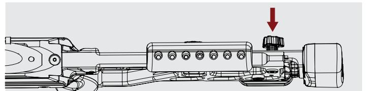
**Step 3:** Move the LOP to desired position and release pressure on thumbscrew.
