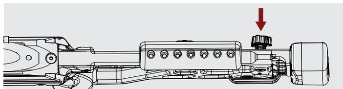
**Step 3:** Move the LOP to desired position and release pressure on thumbscrew.
