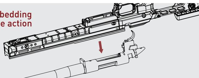
**Step 3:** Drop the rear action screw with washer into the hole just behind the trigger guard, turn the screw to engage the threads in the action. Again do not fully tighten.
