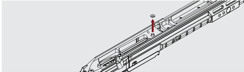
**Step 2:** With the chassis upside down, set your the chassis' bedding area (V-block for Tikka and Radiused area for Remington) onto the action. Turn the front action screw to engage the threads in the action to draw the action into the chassis, do not fully tighten at this point.
