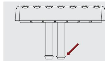
**Step 3:** Optional – You can move the cheek piece forward and backward by removing the two screws holding the cheek piece to the two cheek riser posts and then switching the holes in which the riser posts sit. (use 3mm hex wrench)
