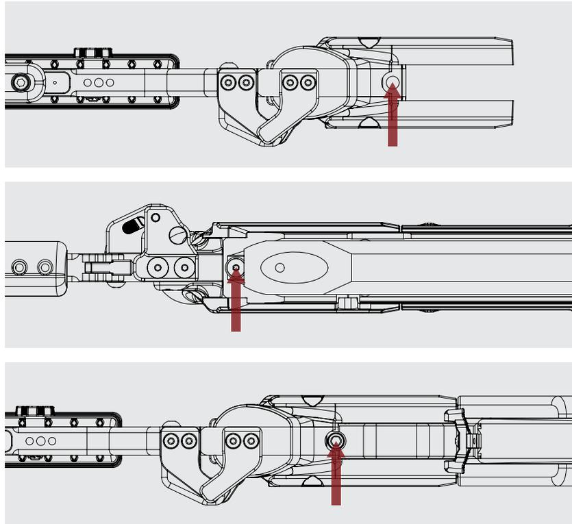
**Step 4:** Tighten the top retaining screw fully.
