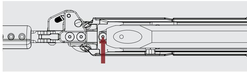
**Step 5:** Tighten the screws on the grip panels, be careful not to over torque these, they are simply holding the polymer panels in place.
