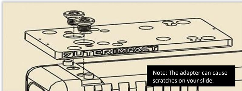
**Step 5:** Using the screws/pins and the mounting pattern identified, mount the Red Dot sight adapter and torque to 12 in/lbs
