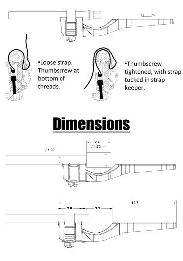
Disclaimer: The bayo is designed to fit tapered and bull barrel muzzles between 0.50 and 1.00 inches in diameter. It is the responsibility of the user to make sure that the bayo is mounted correctly with the sensor deck away from the bullet path.
