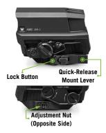
4. To adjust the tension, move the lever back to the open position. Using a flat-head screwdriver or similar device, turn the adjustment nut (pictured) left or right to loosen or tighten (left-looser, right-tighter). Make small adjustments of one or two clicks, then check lever closing tension. It may be necessary to repeat this process a few times until proper tension is achieved.
