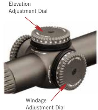
The Razor HD 1–6x24 riflescope uses clicks scaled in 1/2 minute of angle measurements (MOAs) so each small click will move the point of impact 1/2 MOA. **Note:** 1/2 MOA equals .53 inches for each 100 yards of distance [14.55 mm at 100 meters].
