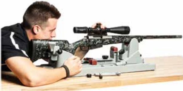
If necessary, make another adjustment and fire another group to verify zero. This procedure can be repeated as many times as necessary to achieve a perfect zero.
