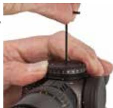
Re-install the cap, aligning "O" mark.
