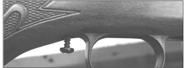
Figure 17B: Rear trigger guard screw of the Savage® 110 serves only to hold the trigger guard to the stock.
