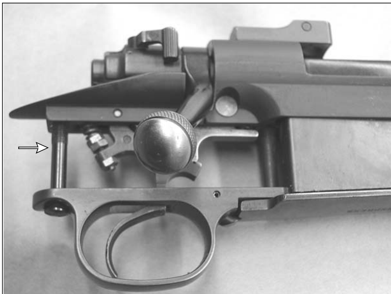
Figure 16D: Rear guard screw is very close to trigger assembly.
