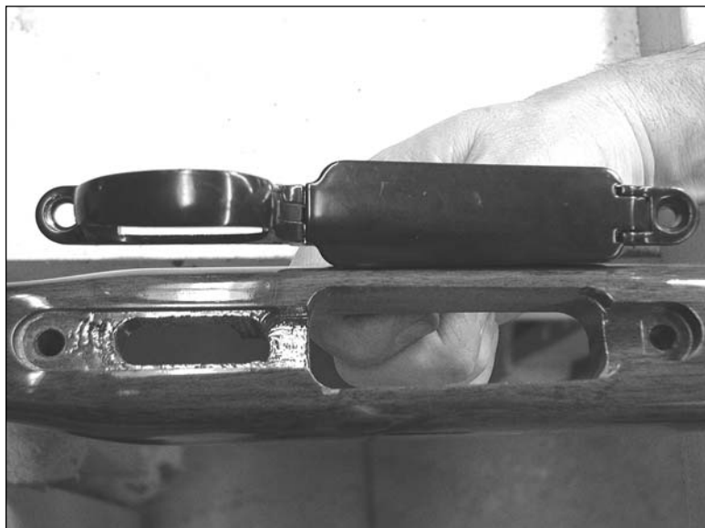
Figure 1F: Bedding the bottom metal can help to support those components in the stock.
