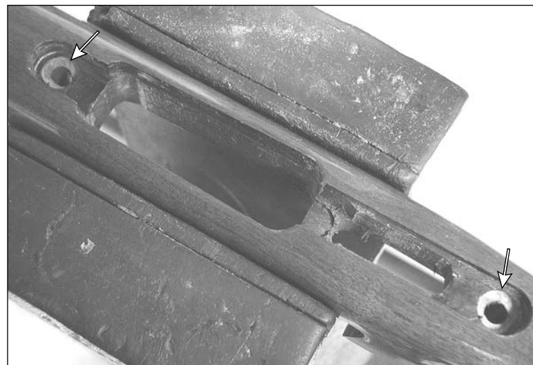
Figure 9B: Guard screw holes enlarged.
