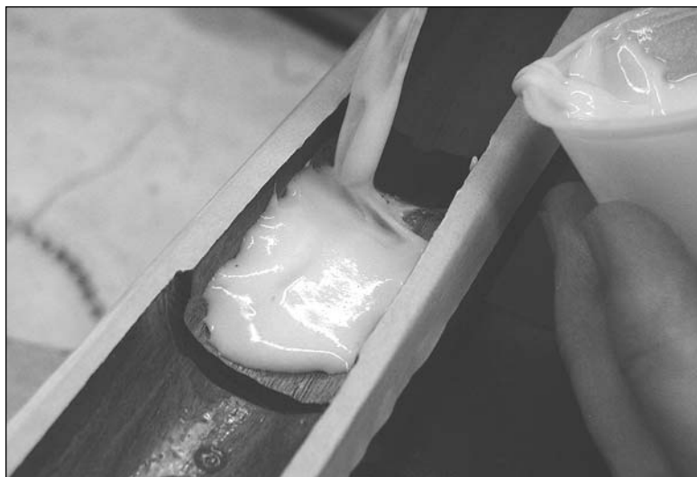
Figure 11A: Transfer Bedrock™ carefully to the relieved areas.
