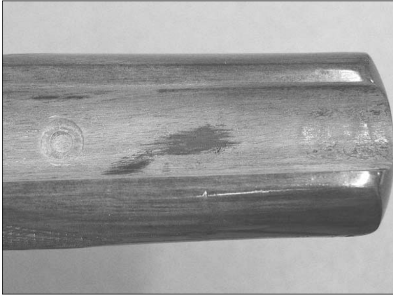
Figure 8B: Inletting black transfers to contact points.
