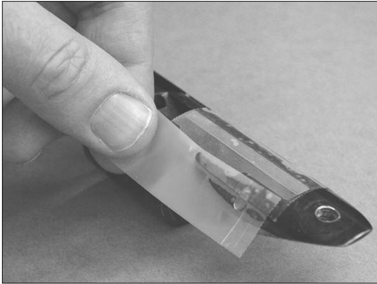
Figure 10A: Plugging or covering holes will keep Bedrock™ from entering the receiver.
