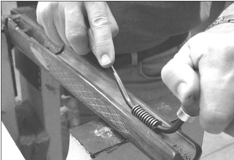
Figure 8C: Removing high spots.
