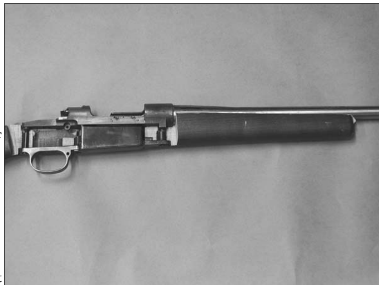
Figure 4Aa: When the rear tang is inletted too deeply, the barrel tends to angle upwards.
