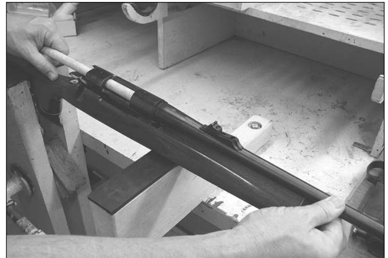
Figure 12A: Lift the barreled action straight up and out of the stock.
