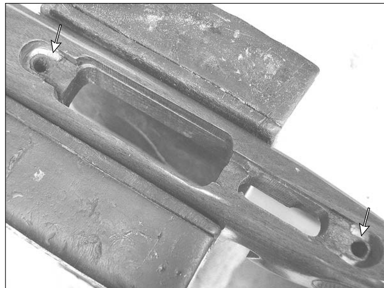
Figure 9A: Outline relieved under trigger guard.
