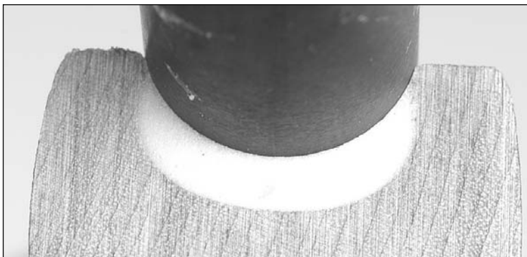
Figure 8: Crossection of stock with hidden bedding.
