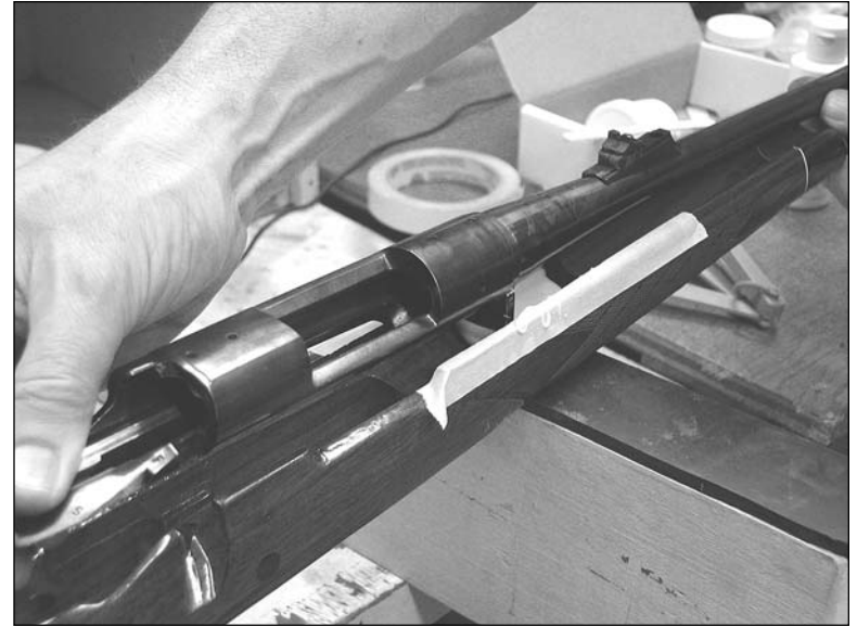
Figure 11B: Carefully lower barreled action into stock.
