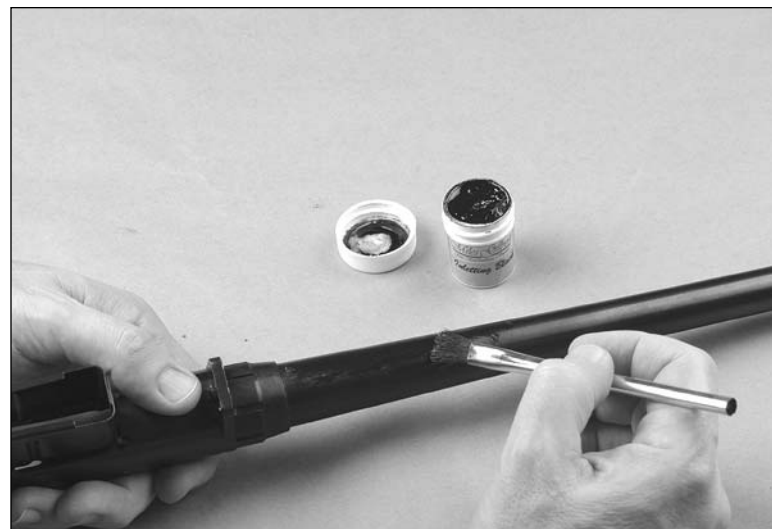
Figure 8A: Applying inletting black
