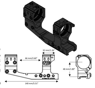
hardcoat anodized. The Torx 20 ring and clamping screws are zinc-nickel coated for corrosion resistance and come pre-waxed from the factory to ensure proper torque values. The mount is shipped with a manual and a "wedge" leveling key.
