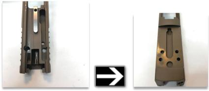
Step 2: Place Outerimpact plate onto slide.
