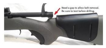
2. Position the adjustable cheek piece sleeve over the butt stock cheek area.
